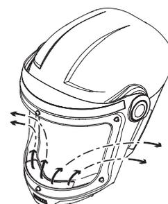
Increased air flow volume creates the required excess pressure inside the hood which prevents overspray intrusion.
